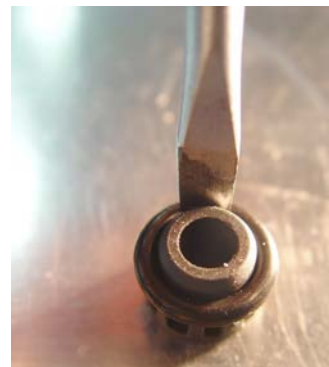
O-Ring in correct position
